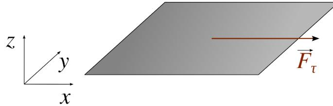
Figure 0.4 – Shear force exerting on a plate
