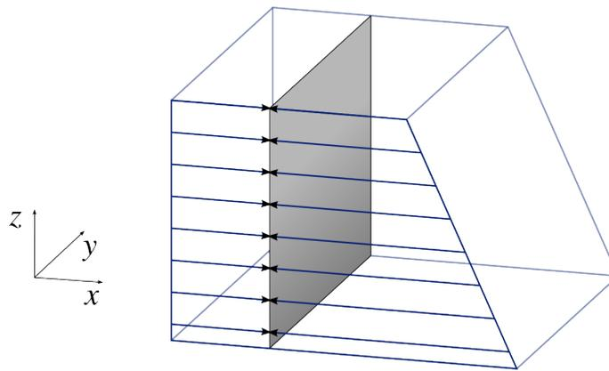
Figure 0.3 – Pressure distribution on a flat plate
