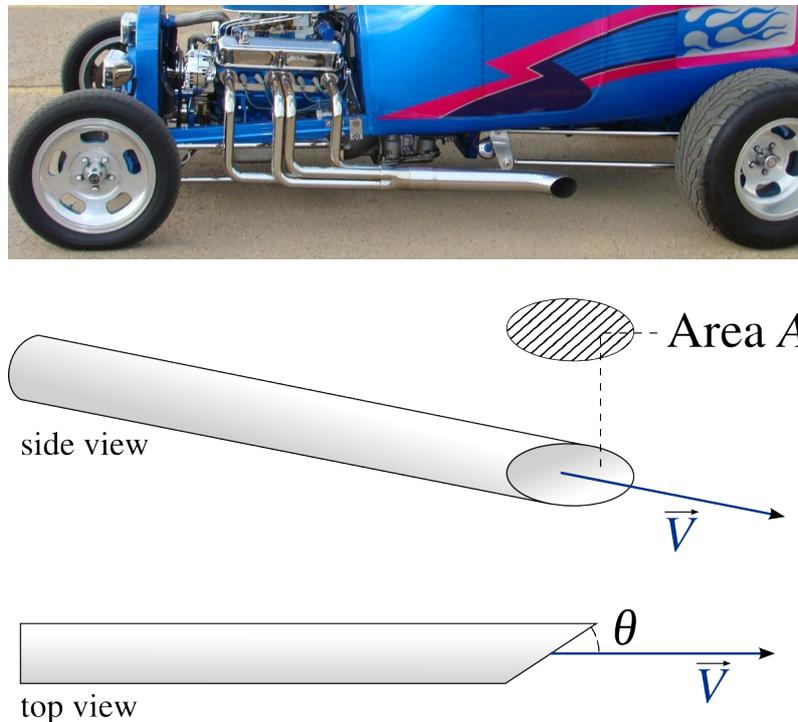
Figure 0.6 – Exhaust gas pipe of a car. The outlet cross-section is at an angle  $\theta$  relative to the axis of the pipe.
