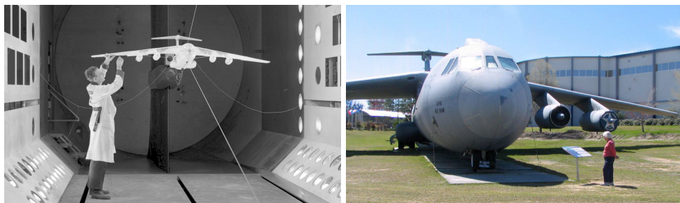
Figure 6.1 – In order for the flow around a wind tunnel model to be representative of the flow around the real-size aircraft (here, a 48 m-wide Lockheed C-141 Starlifter), dynamic similarity must be obtained. The value of all flow parameters must be kept identical. This is not always feasible in practice.
