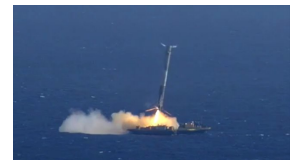
Video: rocket landing gone wrong. Can you compute the moment exerted by the top thruster around the base of the rocket as it (unsuccessfully) attempts to compensate for the collapsed landing leg? by Y:SciNews (STYL) https://youtu.be/4cvGGxTsQx0
